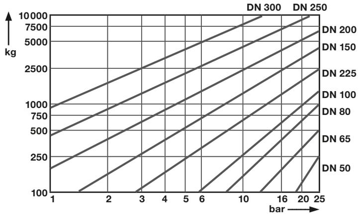
Pressure thrust forces of ERV Expansion Joints
